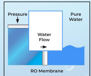
High pressure forces water through the semipermeable reverse osmosis membrane element. RO membranes are made of a thick polyamide film that contains tiny pores through which water can flow.
